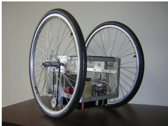
Fig. 1.14 QUASIMORO, a quasiholonomic mobile robot
